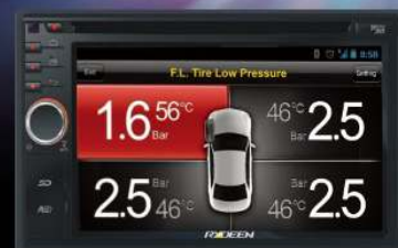
DVA6 screen showing Tire Pressure Monitoring System (Model TPM1)
